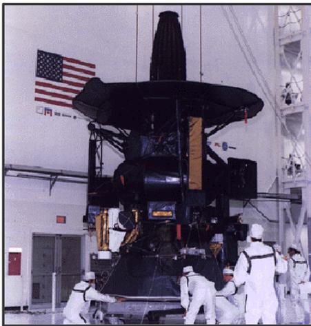
**Fig. 10-8 NASA Galileo Spacecraft with two nuclear powered generators**
