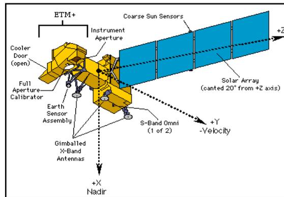
**Fig. 10-10 LANDSAT with earth and star sensors**
