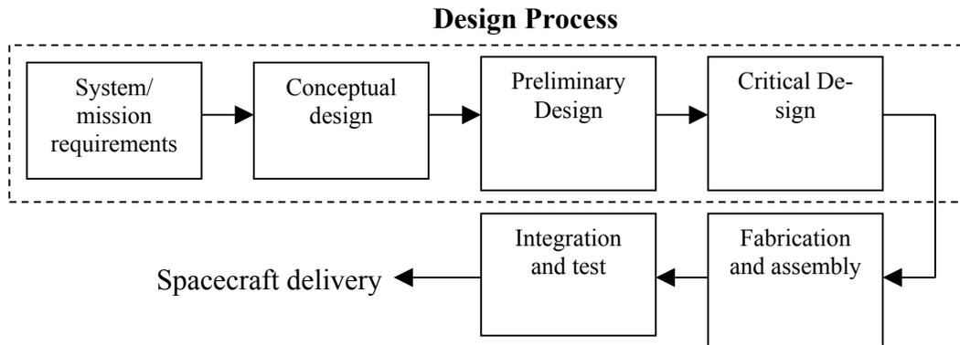
**Fig. 10-1 Spacecraft design phases**
