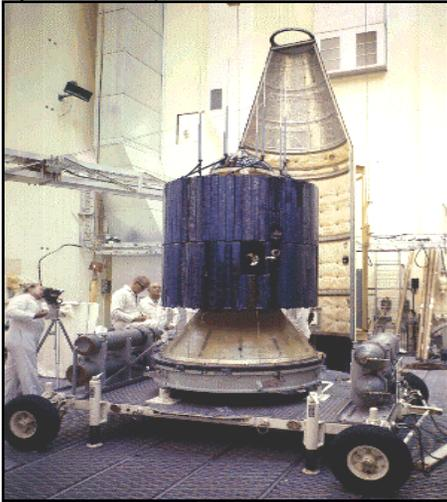
mass and cost, and Fig. 10-3 Satellite being fitted to rocket faring
