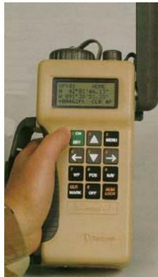
**Fig. 14-9. Hand-held Precision Lightweight GPS Receiver (PLGR)**
