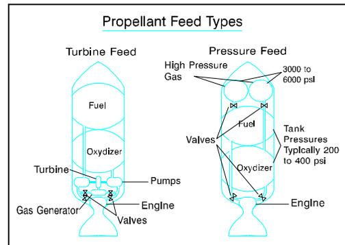
**Fig. 5-8. Propellant Feed Types**
