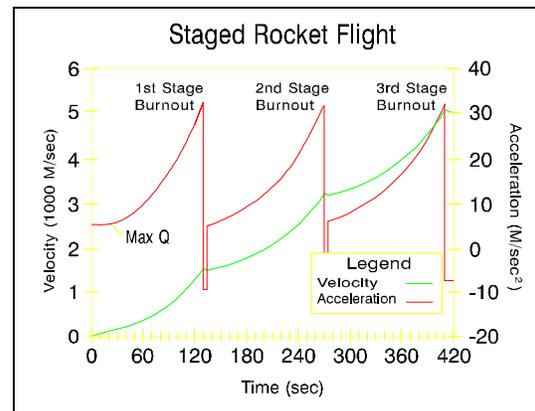
**Fig. 5-2. Acceleration and Velocity**
