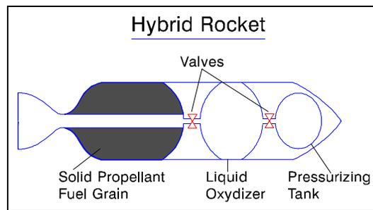
**Fig. 5-11. Hybrid Rocket System**
