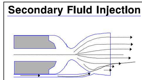
**Fig. 5-17. Thrust Vectoring**
