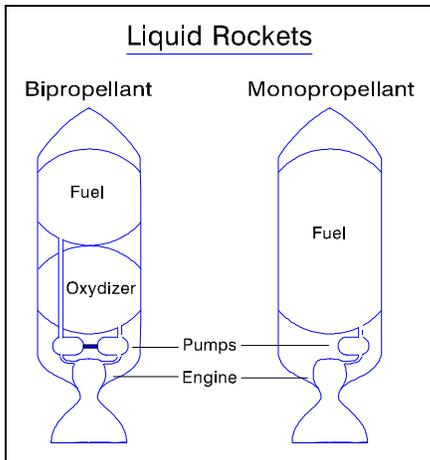
**Fig. 5-7: Liquid Propellants**
