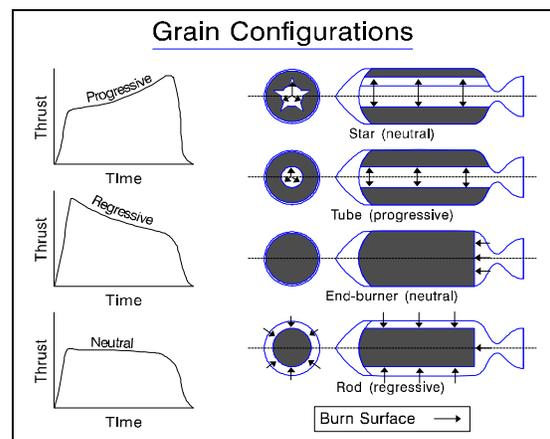
**Fig. 5-10. Grain Configurations**
