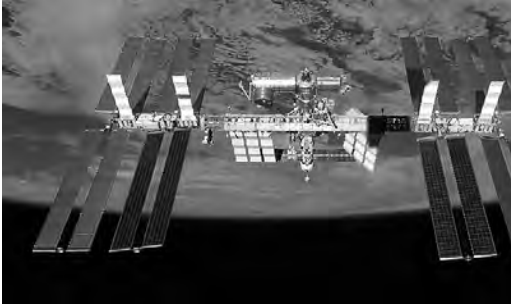
Figure 22-5. International Space Station with large deployable solar arrays. (NASA photo)
