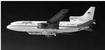
Figure 20-5. Orbital Sciences Corporation L-1011 Pegasus launcher. (NASA photo)
