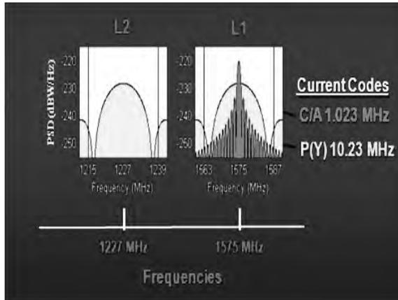
**Figure 16-1. Signal/frequency/code relationship.**
