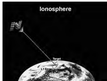
Figure 16-3. Error induced on L1 by the ionosphere. (NSSI graphic prepared by the author)
